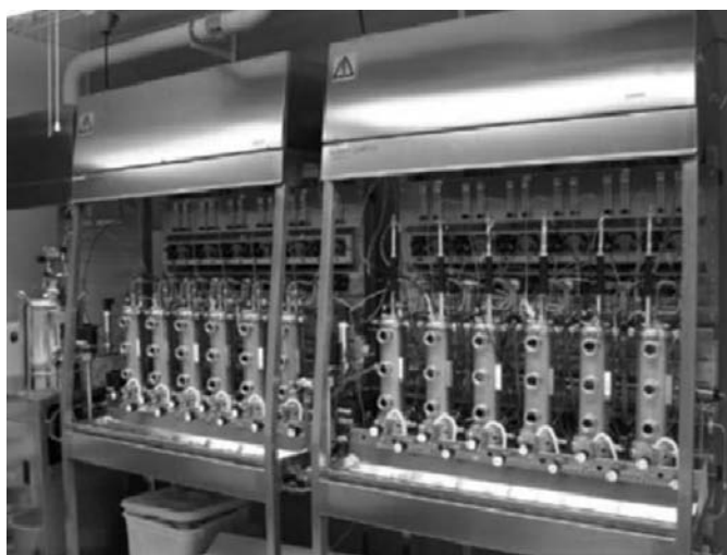
Figure 1 The bioprocess unit of GRETA, encompassing 12 fermentation chambers.
